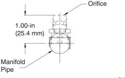
Fig. 32 - Orifice Projection
